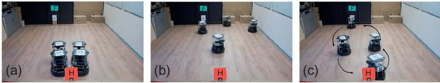
**Figure 13.9** Multi-robot foraging using swarm robots with extended resources. (a) All robots start at the hive (H) location. (b) Robots are exploring the unknown environment randomly. The left two robots have found the food (F) location and are foraging between the hive and the food location. (c) All robots have converged to foraging behavior.
